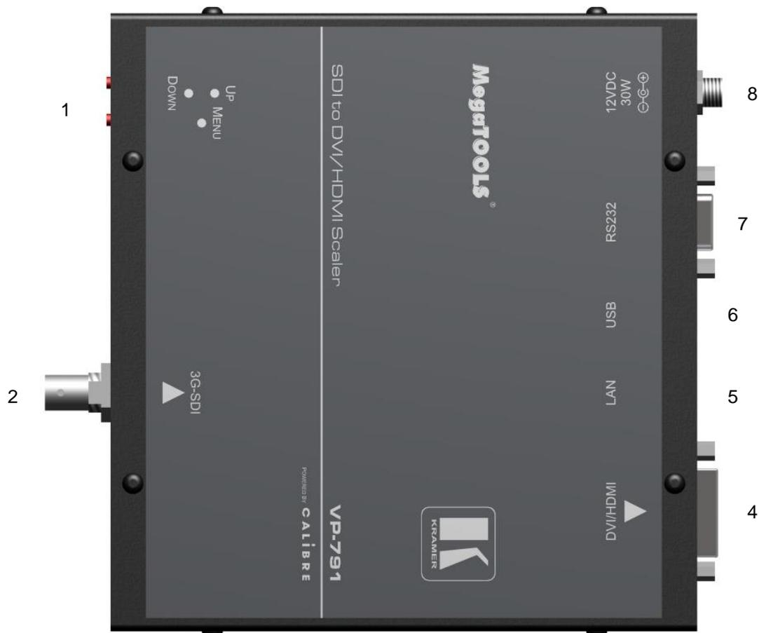
1 – Keypad with three keys for OSD menu navigation (Menu, Down and Up).
