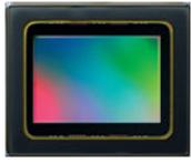
The large 1.0-inch, 20.1 Megapixel\* CMOS sensor helps capture high-quality images and videos with a wide dynamic range, a high resolution for detailed prints
