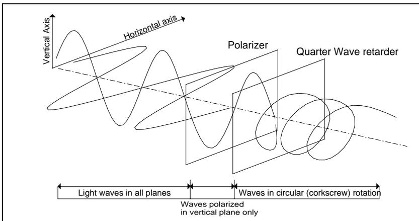
From the left the light waves are in all planes. When they reach the polarizer only the waves in the vertical plane can pass. When they reach the quarter wave retarder they are slowed down by 90° producing a cork screw type of polarization.
