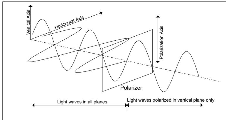
From Malus's Law the maximum level of light which can pass through a polarizer is 50%. Formatt filters are HN38 polarizers, meaning that a maximum of 38% can pass. This equates to 1 1/3 stops and suitable adjustments should be made. Formatt uses a very high specification iodine tinted polymer for its polarizers, ensuring a neutral grey with a flat transmission curve, minimising the risk of any colour distortion.
