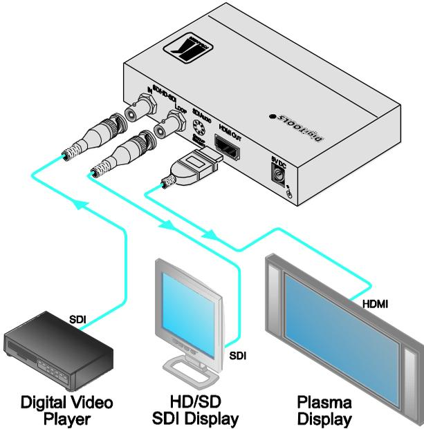
Figure 2: Connecting the FC-331 SD/HD-SDI to HDMI Converter
