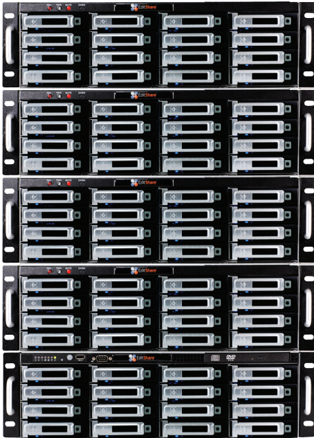
XSTREAM 3U Workflow director and four expansion chassis.
