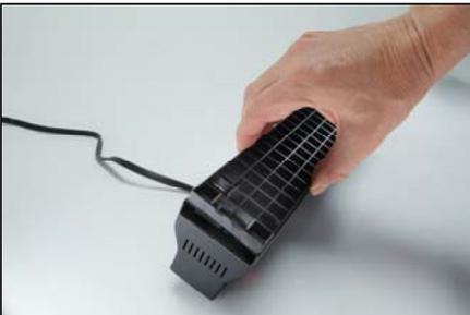
Insert the Louver to hold the gel in place.
