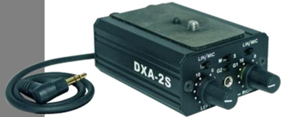
*The BeachTek DXA-2s is a two channel, transformer balanced XLR adapter for today's small, compact camcorders. This adapter is designed to easily attach balanced or unbalanced type microphones to any camcorder with a MIC jack. The DXA-2s gives you all the benefits of using balanced audio devices for clean audio as well as control over the signal levels to ensure the best possible sound recording.*
