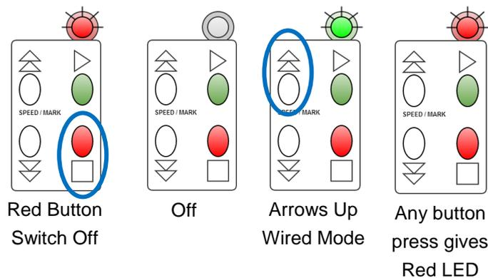
**iOS users:** When in wired mode the remote sends DTMF tones to the cell phone or tablet. Please allow the permission for the App and remote to use headset or microphone input.
