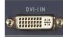
The advanced connection options include DVI-I making it easy to connect to computer equipment.
