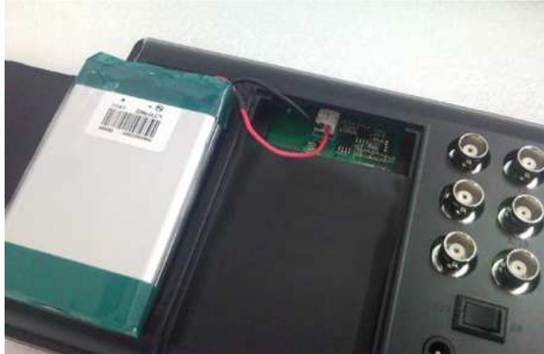
4 . Put the battery into slot when check the electricity.
